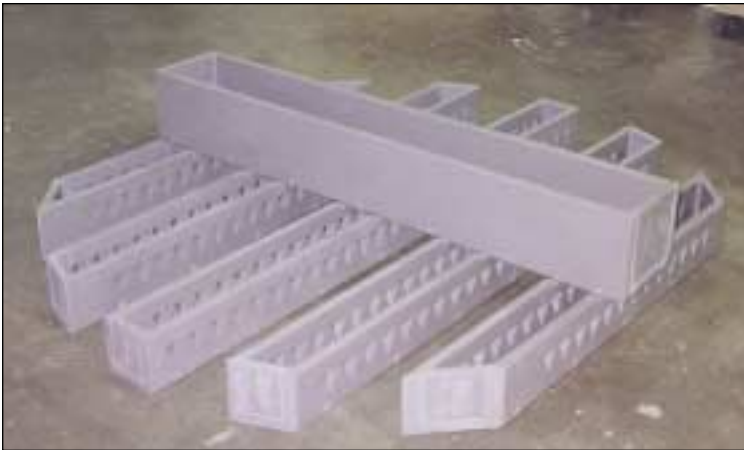
Corzan™ CPVC weir trough distributor with elevated parting box, utilizing triangular weirs for flow distribution. Good for fouling services and turndown capabilities.
