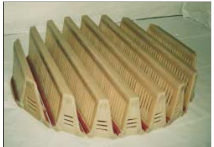
PVDF 84" diameter, gas injection packing support plate with high open area. Support plate utilizes 2" PVDF pipe with encapsulate FRP rod for added rigidity.
