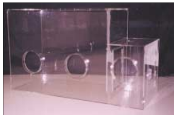
Acrylic glove box with transfer chamber
