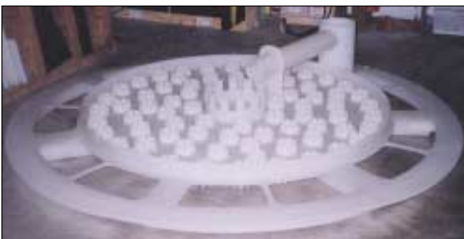
PVDF eight-foot diameter, liquid distributor designed to rest between tower body flanges. Distributor is fabricated with slotted weir down pipes and wipe vapor passages near the flanges.
