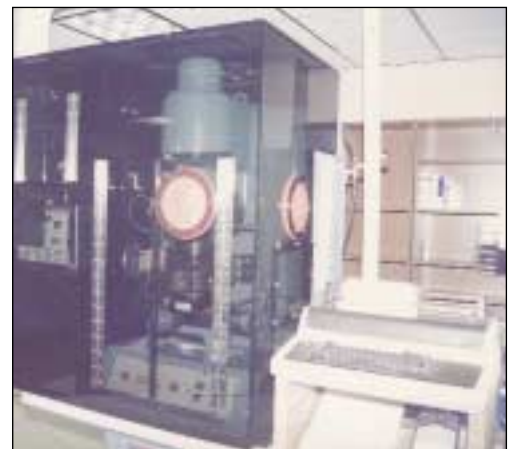
Smoked acrylic instrument enclosure with glove ports
