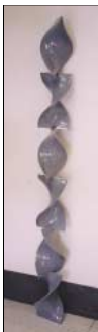
Motionless mixing pipe insert fabricated from CPVC sheet
