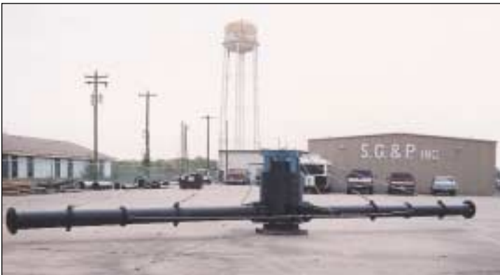
Polyethylene rotary trickle distributor, used in a bio-pond application as an alternate to the aluminum one which had failed in service
