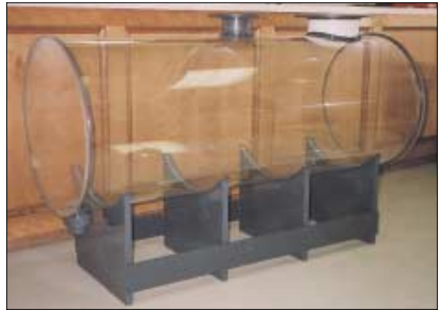
24" diameter acrylic tank, with PVC stand
