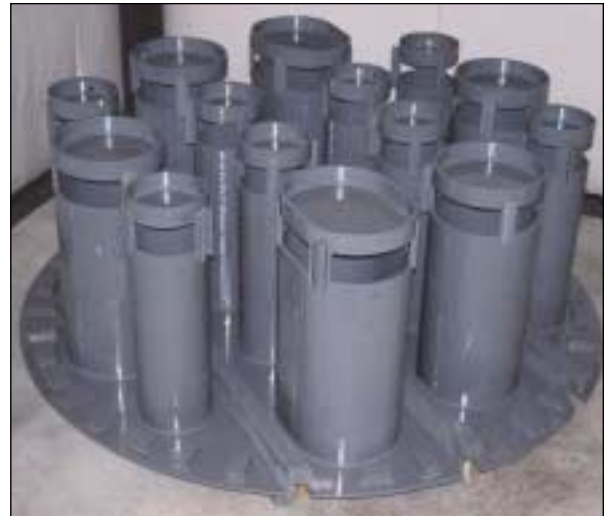
Corzan™ CPVC chimney tray for liquid collection and draw-off. Contains multiple vapor risers for equal vapor distribution.
