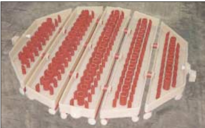
PVDF liquid redistributor with vapor risers and angled drip tubes. Sectional construction incorporates lateral cross flow tubes for liquid transfer.
