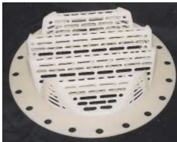
PVDF three-foot diameter, gas injection type packing support designed to fit between tower body flanges and also designed for a high open area.
