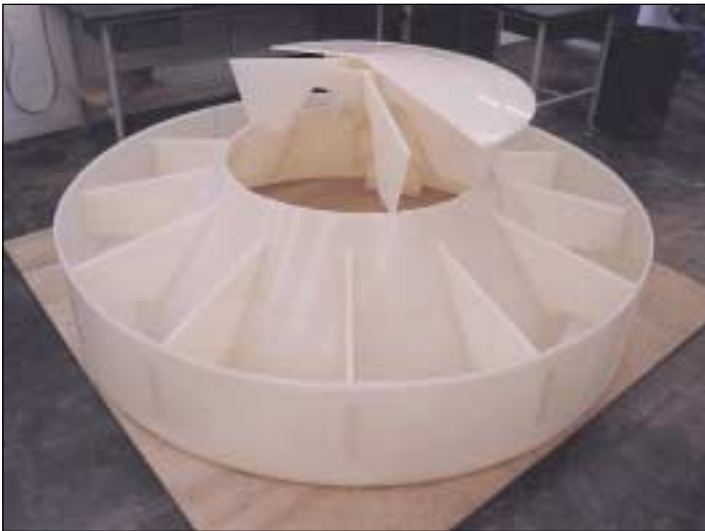
PVDF eight-foot diameter, single vapor riser liquid collector, with welded PVC wall wiper for total liquid drain-off. Designed for critical service requiring zero liquid leakage. Collector was piece welded inside the tower using S.G. & P. field services.
