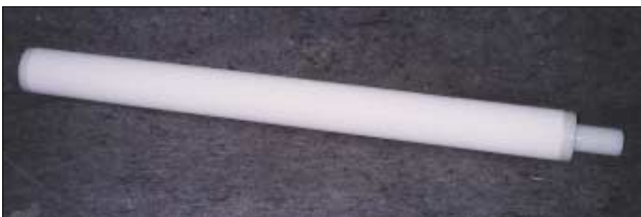
Porous HDPE filter element fabricated from porous HDPE tube and HDPE rod for the threaded end and end caps, using butt fusion technique
