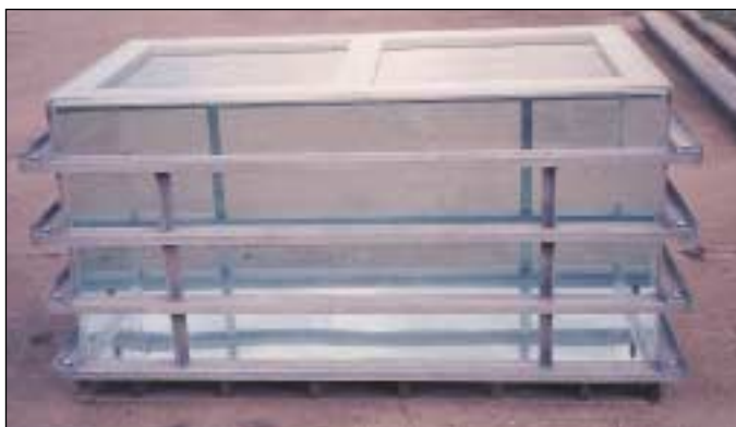
Large acrylic tank with metal support frame
