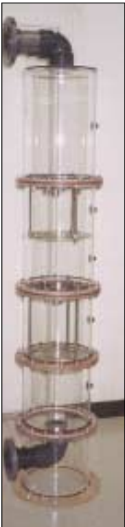
12" diameter acrylic flanged column with PVC flanged connections
