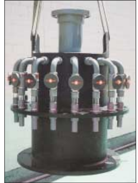
Radial liquid distribution unit fabricated from polypropylene sheet, CPVC pipe and fittings and enclosed in a custom fitted stand fabricated from polyethylene pipe and sheet
