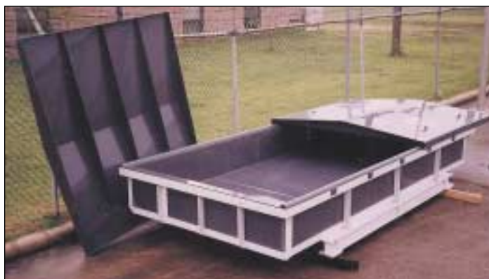
PVC vat with sliding covers in a metal frame
