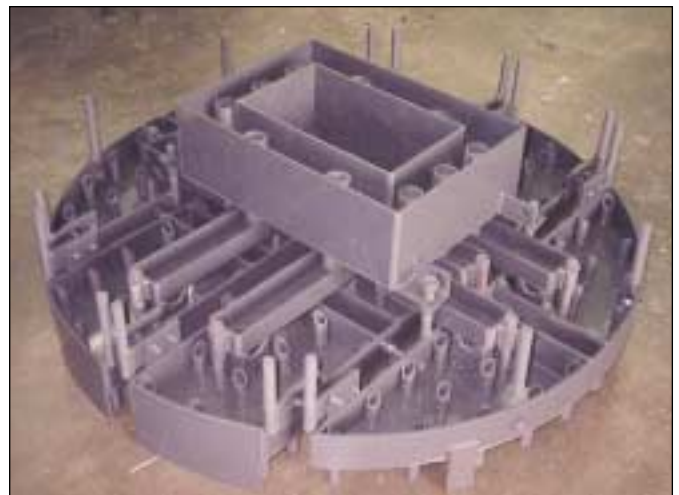
MTS-109 PVC distributor, fabricated under exclusive license with Nutter Engineering from Dow Chemical. Sectional design minimizes out of level effects. Angle drop tubes provide flexibility in turndown situation.
