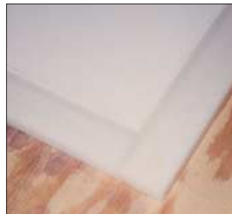
Porous HDPE filter plate, ten feet long with solid HDPE sheet welded on as a frame with o-ring grooves routed on the face of the frame
