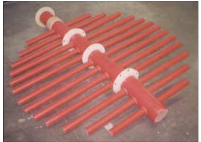
PVDF pipe-arm (ladder-arm) type distributor. This type distributor can be fabricated for use in liquid or vapor applications. It can also be fabricated with fitted spray nozzles.
