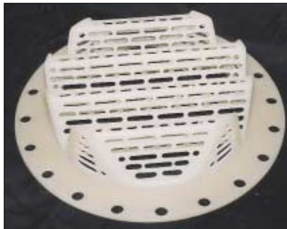
PVDF three-foot diameter, gas injection type packing support designed to fit between tower body flanges and also designed for a high open area.
